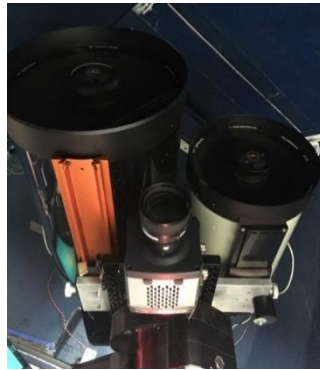
The telescope system used to collect the data: an Andor NEO camera, 85 mm F1.4 Nikon lens
